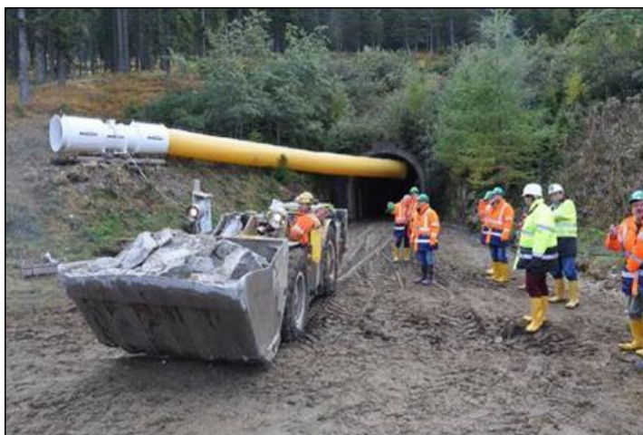
Figure 5-3: Photograph of bulk sampling being carried out by European Lithium in 2013 Source: European Lithium
