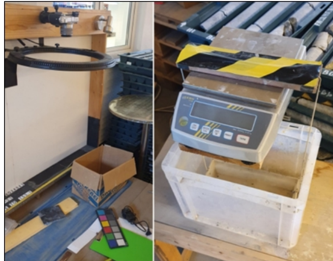
Figure 9-5: Core photography rig (left) and density station (right) at the Wolfsberg core processing and storage facility Source: CSA Global
