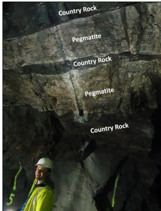
Figure 9-9: Pegmatite exposure in the roof of an exploration drift; note the internal country rock and channel sample Source: CSA Global
