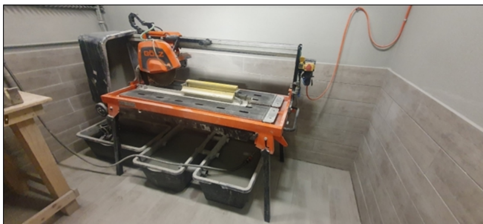
Figure 9-6: Core saw at the Wolfsberg core processing and storage facility Source: CSA Global
