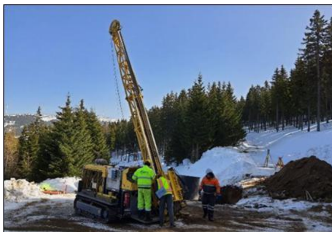
Figure 7-6: GEOPS rig drilling hole P18-09 as part of the 2021 drilling program Source: European Lithium/DRA
