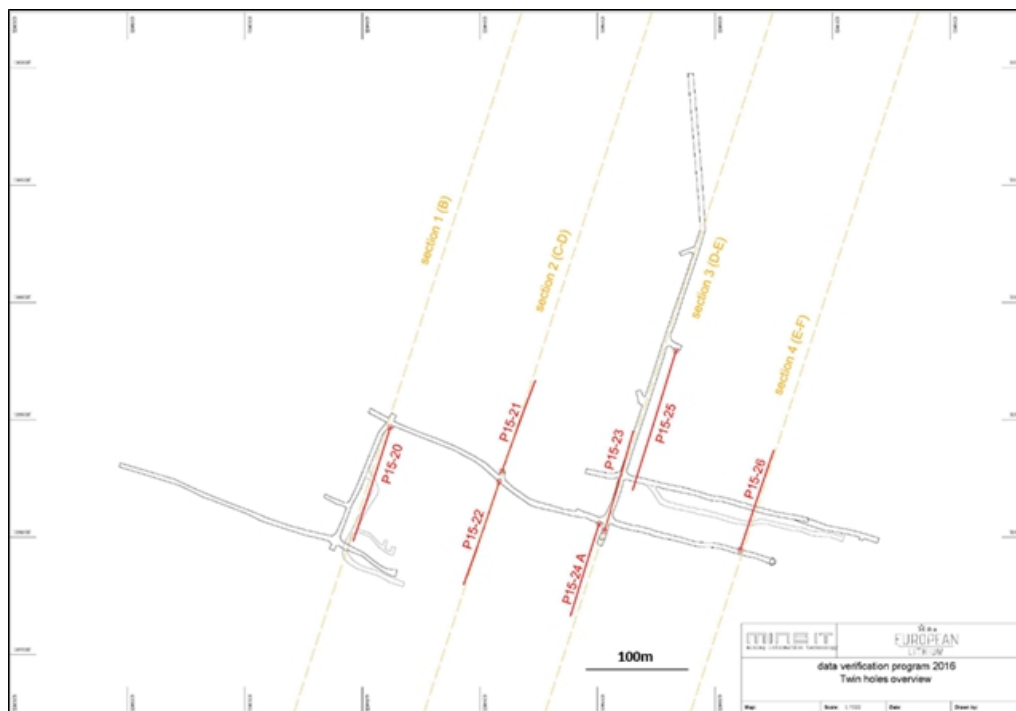
Figure 7-3: Overview map with underground workings and drillhole locations from the 2016 underground drilling
