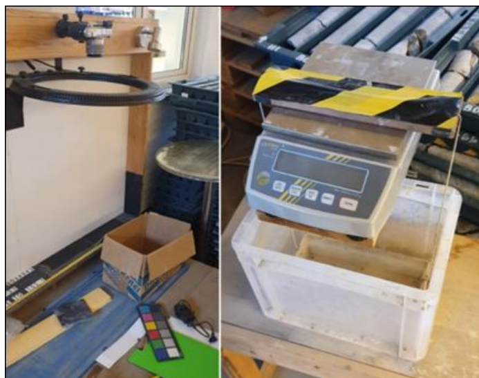
Figure 9-5: Core photography rig (left) and density station (right) at the Wolfsberg core processing and storage facility
